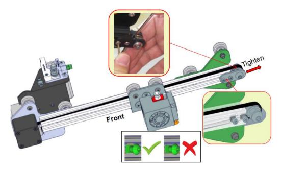
**Step 1.** Prepare belt tensioner assembly (K1) and 3mm Allen key.
