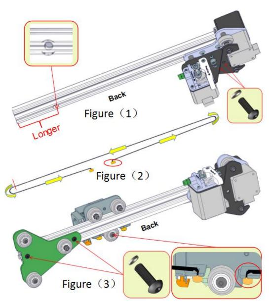
**Step 1.** Assembly of aluminum profile (B1) and extrusion assembly (E). Aluminum profile (B1) is shown in the diagram on the left(1). Pay attention to the position and direction of the large hole. Align the hole of extrusion assembly (E) with the threaded hole of aluminum profile (B1), it should be noted that the hole has two plates, which are secured with M4\*16 screws, and fixed to the second profile plate and the aluminum profile (B1). Use the Allen key to tighten the screws.
